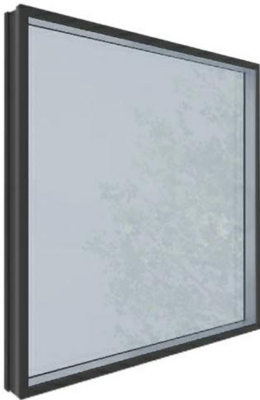
GL-1 1" INSULATED VISION GLASS GLASS TYPE: SUNGUARD 51/23 ON CLEAR NEUTRAL BLUE APPEARANCE VLT: 51% SHGC: 0.23
